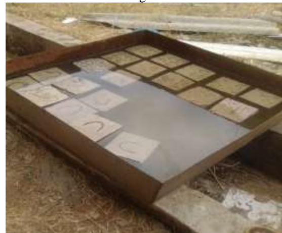
Plate 2.3: Curing of concrete cubes
